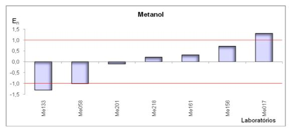
Figure 13 – Performance evaluation by normalized error - Methanol analyte
