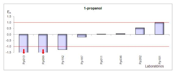
Figure 17 - Performance evaluation by normalized error - 1-propanol analyte
