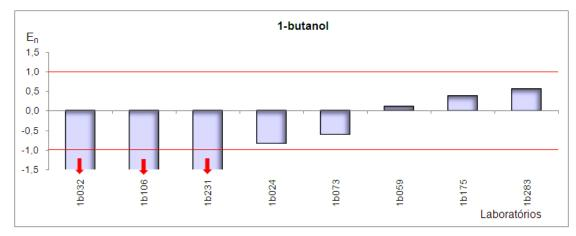
Figure 14 - Performance evaluation by normalized error - 1-butanol analyte
