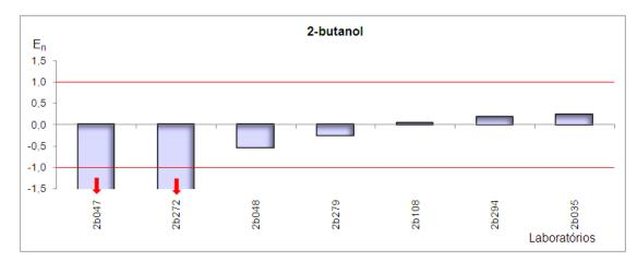
Figure 15 - Performance evaluation by normalized error - 2-butanol analyte
